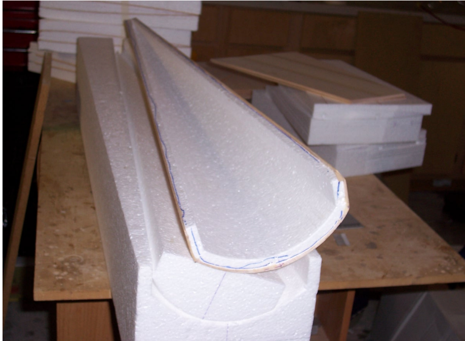
Sheeted Bottom Rear Fuse Deck
