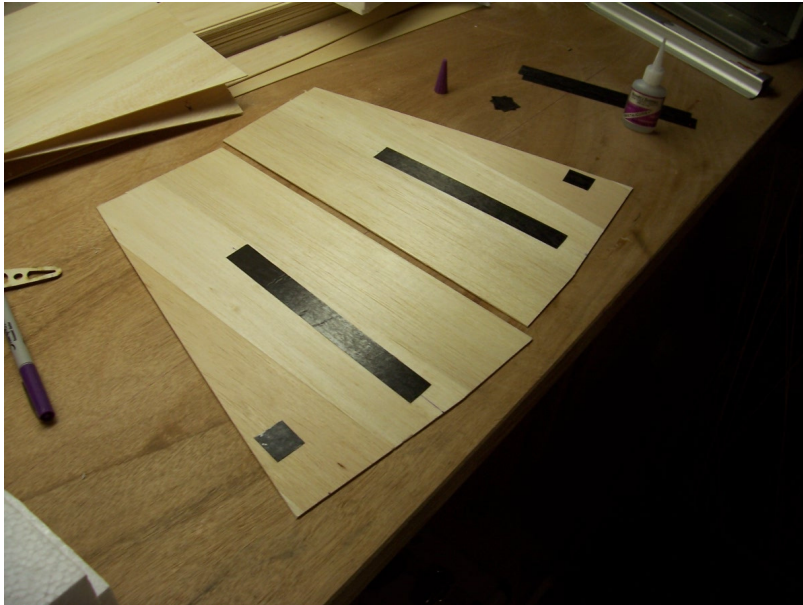
Stab skins with carbon fiber CA'd in place.
