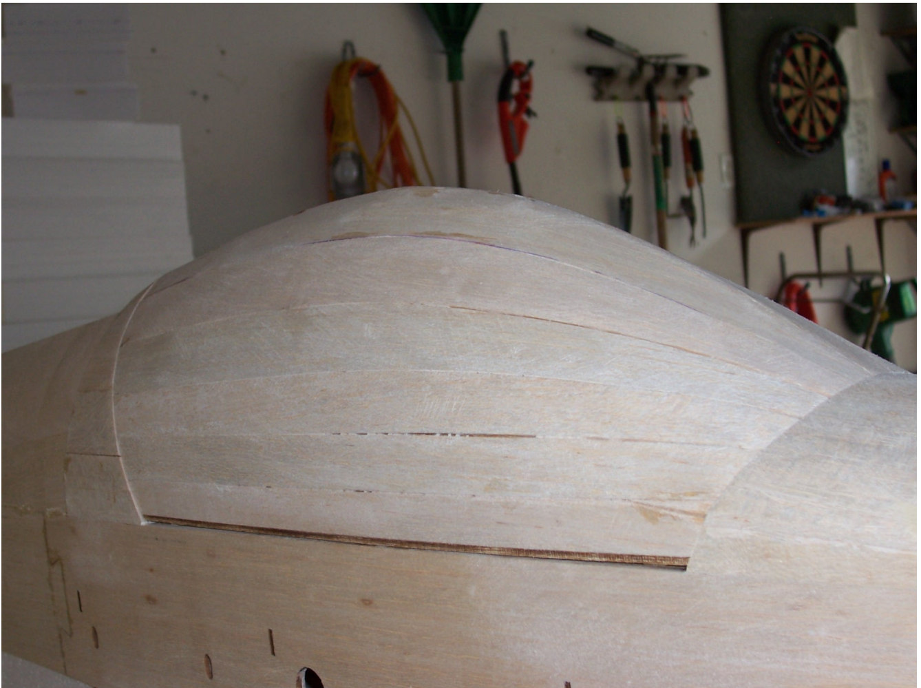
Sheeted ("rough") canopy.
